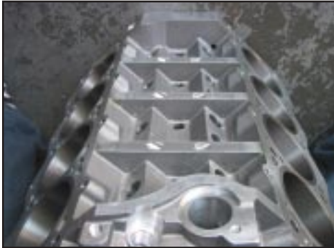
A look at the valley of the aluminum Man O'War block shows the reinforcing ribs and lifter pads. Lifter bores are indexed to assure optimum valve train geometry.
