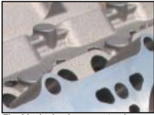
The block also incorporates bosses for lifter cross-feeds (shown) as well as bosses for dry sump oiling.
