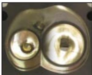
CNC ported combustion chamber and ports designed by Kuntz & Co.
