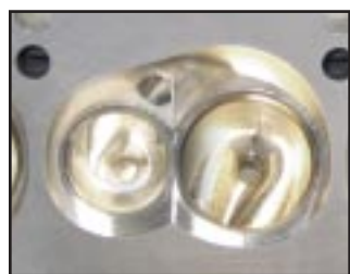
Highly efficient CNC-ported chamber and large valves boost performance
