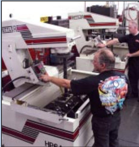
One of the key operations in race-prepping a block is honing the cylinders to the desired specifications using special plates to simulate the loads exerted on the block by the cylinder heads. World employs highly accurate Rottler Power Hones for the task.
