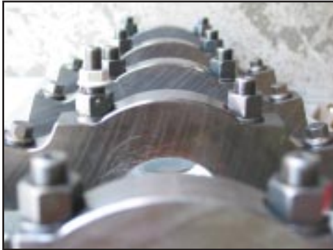
The bottom end of the aluminum Man O'War block is also a study in engineering excellence. Race blocks are equipped with billet steel splayed 4-bolt mains.
