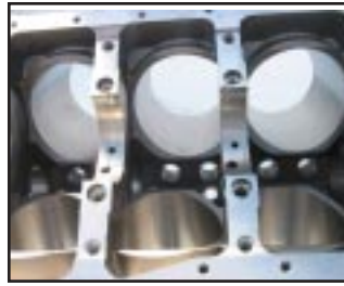
The Man O'War's crankcase is designed to clear a 4.250" stroke crankshaft for big-inch engines.
