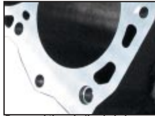
Recessed threads (begin below deck) and blind tapped bolt holes assure proper clamping.
