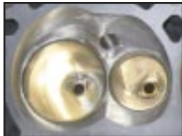
CNC-ported combustion chamber and bowl
