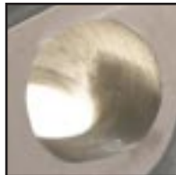
Kuntz & Co designed CNC exhaust port
