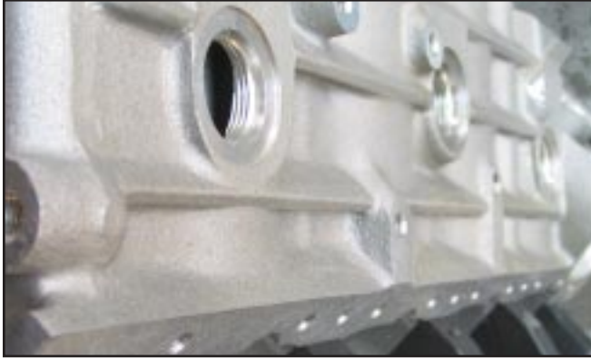
World's ribbed Merlin X block provides extra cooling and outstanding cylinder stability. It also gives the Merlin X a distinctive look.
