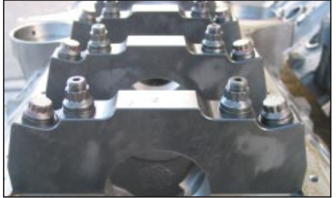
With 4-bolt splayed 1045 alloy billet steel main caps and 200,000 psi ARP® main studs and bolts, superior reliability is assured.
