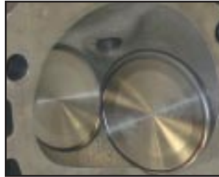
119cc combustion chamber with 2.300" intake and 1.880" exhaust
